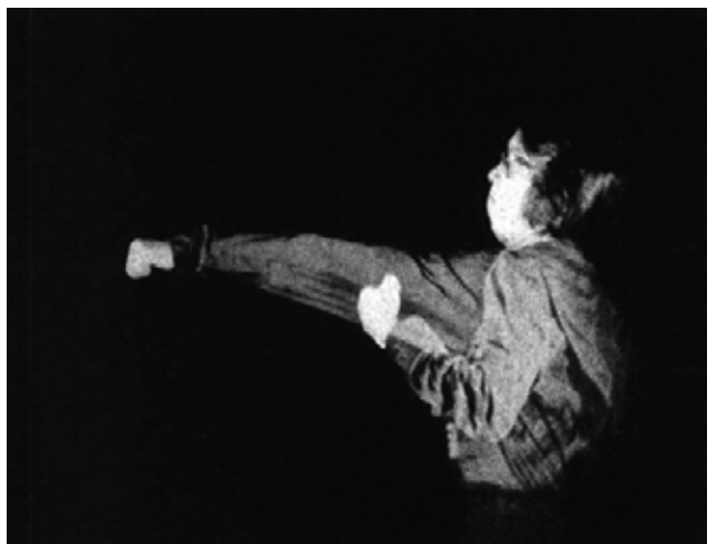
The speed of a punch was also tested. Here we see one interval of 30 flashes per second. Therefore, it takes 0,03 or 3/100 of a second for the punch to be completed.
